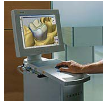
CEREC in-office direct milling system: This represents an adjustable occluder with virtual reality capability and CAD/CAM machining
