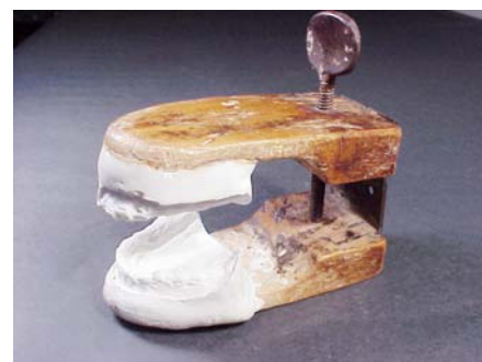
Simple hinge with vertical stop from the Whip Mix Co. historical collection
