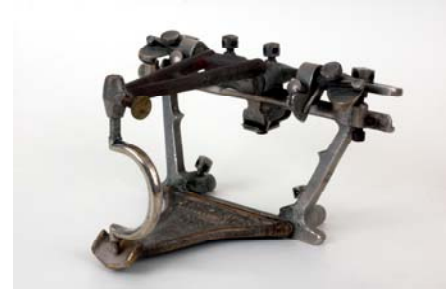
Gysi adaptable instrument: This represents an early adjustable articulator (1912)
